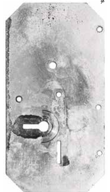
Cover plate of an 8-lever lock.
