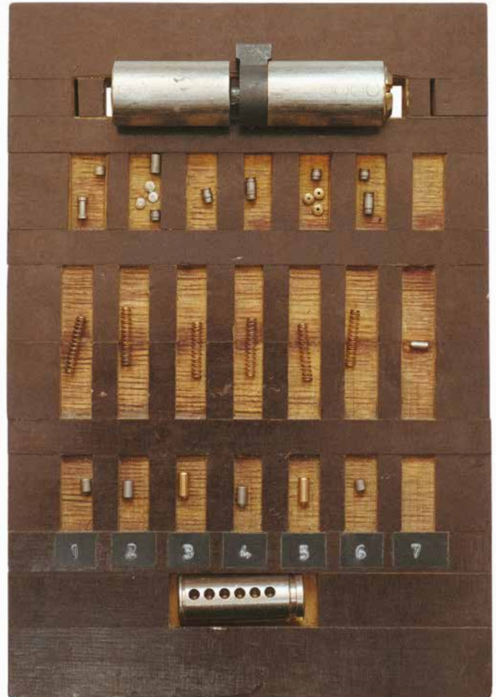
Pinning tray with a gutted 6-pin tumbler lock (master-keyed).
